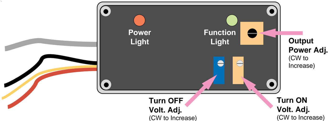
3. With a small straight-slot screwdriver, rotate the screwdriver adjustments on the multi-turn, **turn on** and **turn off** controls fully **counter clock wise** (CCW) 20 full turns. Then rotate the **turn off** control clockwise (CW) two and one half (2-1/2) turns.
